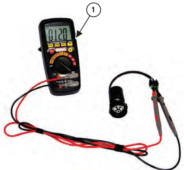
Figure 56: Voltmeter Coil Check
