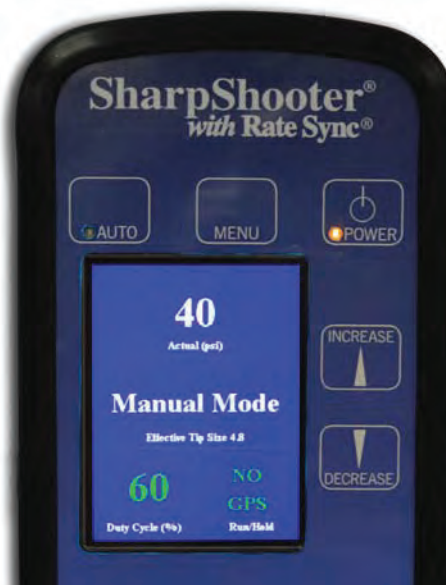
Figure 25: SSRS Display Controls
