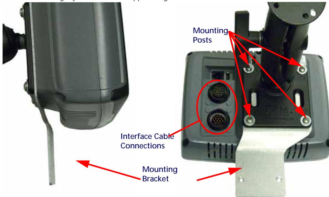
**NOTE:** When mounting the Switch Pro unit with a Viper Pro field computer, the optional Viper Pro mounting bracket (P/N 115-0171-181) can be used to mount the Switch Pro either above or below the field computer.
