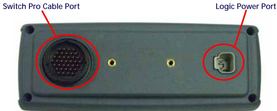
3. Connect the Switch Pro to the existing SCS console cable.
